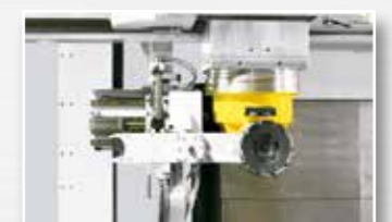
vertical and horizontal automatic tool changer
