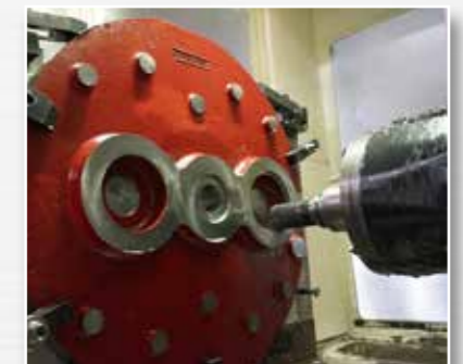
Boring the base
